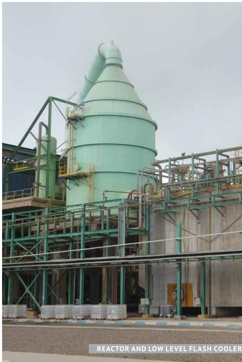
REACTOR AND LOW LEVEL FLASH COOLER
