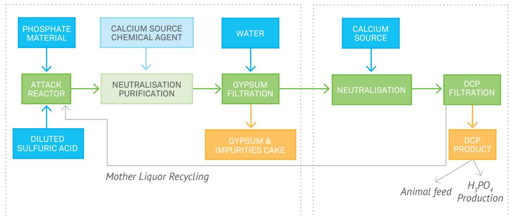
New **Prayon** process produces DCP from low-quality raw materials while using diluted sulfuric acid, a reagent available in any phosphoric acid plant. Impurities are discharged along with gypsum, a common by-product in the phosphoric acid industry that can be stacked following the same environmental rules.
